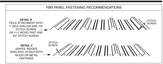
PBR Panel can be used for a variety of different applications. Due to its design, it is a roofing and siding profile. When being used as a siding application, please refer to detail C for fastening. As the height on the sidewall may change the on-center attachment recommended, please consult load chart on page 1.
